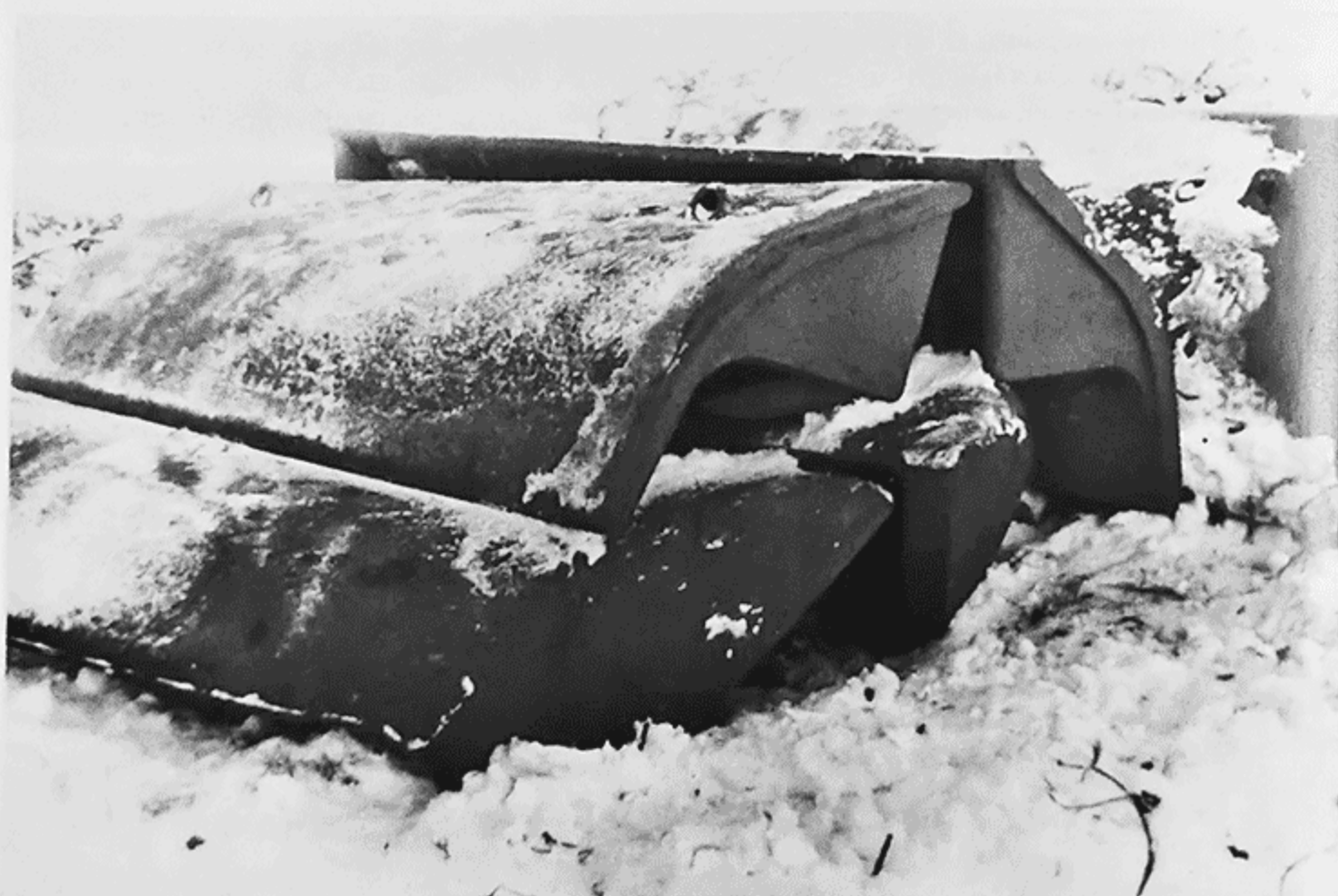
Above and Below: All six sections of the Kettenschutz (track guard) had been delivered and were stored outside when the assembly status report was written in January 1945. (NA)
