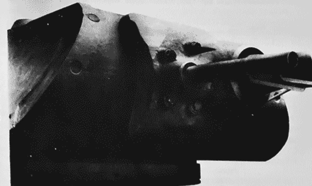
Right: The coaxially mounted 7.5 cm Kw.K.44 L/36 also shared the same cast gun mantle as the 12.8 cm Kw.K.44 L/55 . (KSM)
