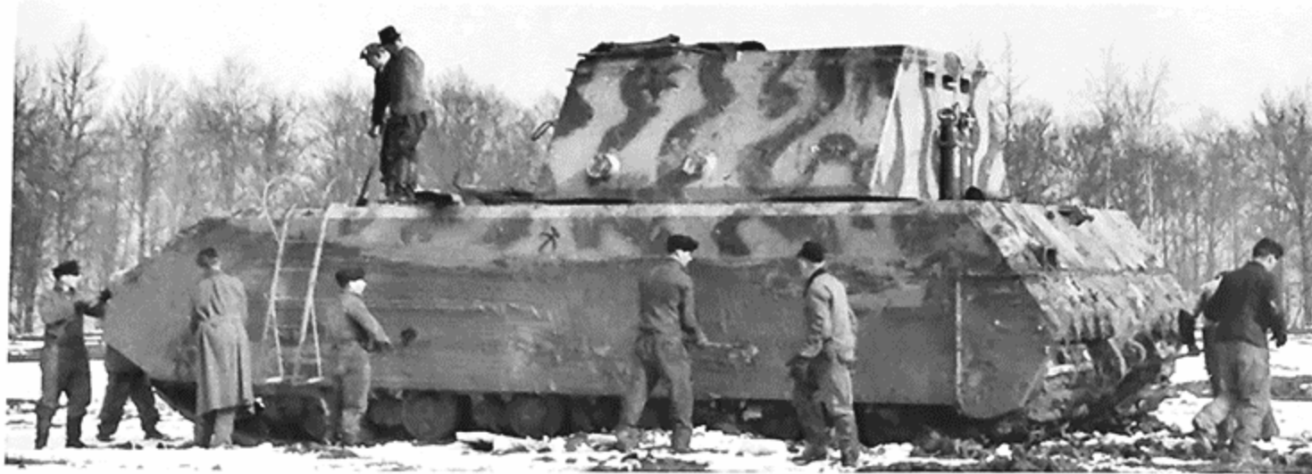
Above and Below: The I.Maus chassis became stuck during a trip through a swampy area because the driver didn't know the area (a region avoided by lighter Panzers). After the mud churned up at the rear was dug out and timbers laid under the tracks, the Maus pulled free under its own power. (TTM)
