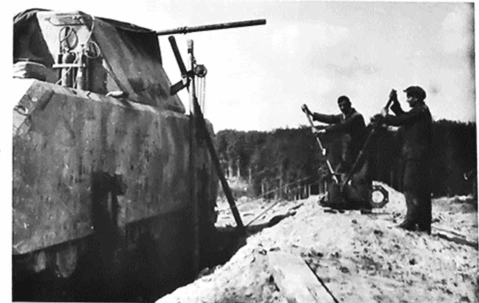
Left Below and this Page: As reported on 20 March 1944, the I.Maus was jacked up to install the improved roadwheels. The drive train components such as the engine, generators, electrical motors, final drive with brakes, and the differential were taken out and dismantled for inspection. (WJS)
