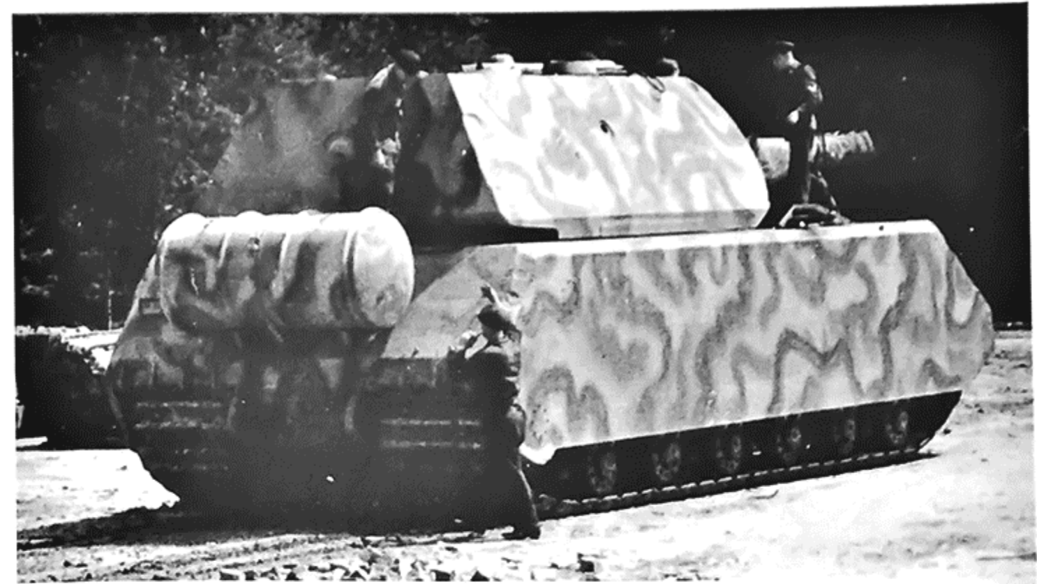
Above: After being sprayed with camouflage paint (base coat of Dunkelgelb RAL 7028 with Olivgruen RAL 6003 and Rotbraun RAL 8017 stripes), the complete Maus Versuchs-Fahrzeug (Fahrgestell Nr.2 and Turm Nr.1) still had roadwheels with holes drilled in the pressure discs. (WJS) Below: These roadwheels had been replaced before this Wa Pruef 6 photo was taken. (WJS)
