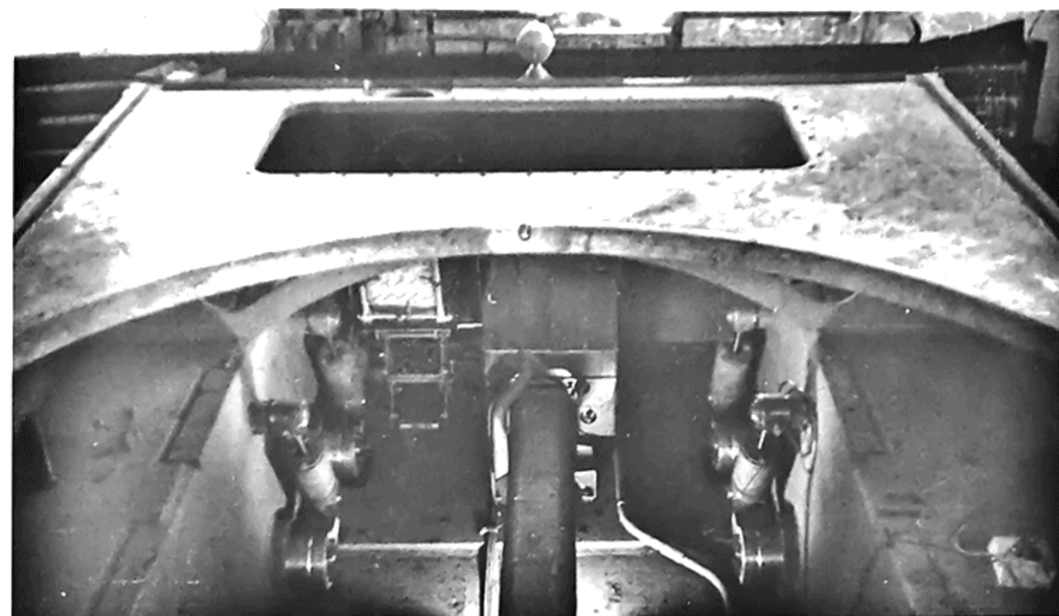
Above: The front deck with the cutout for the missing Abdeckplatte (cover plate with the driver's and radio operator's hatches). Inside, two shock absorbers are located on each side with the covered transmission and main drive shaft cover in the middle. Below: Curved segments were cut out of the inside surface of the hull sides to gain clearance for the turret platform. (NA)
