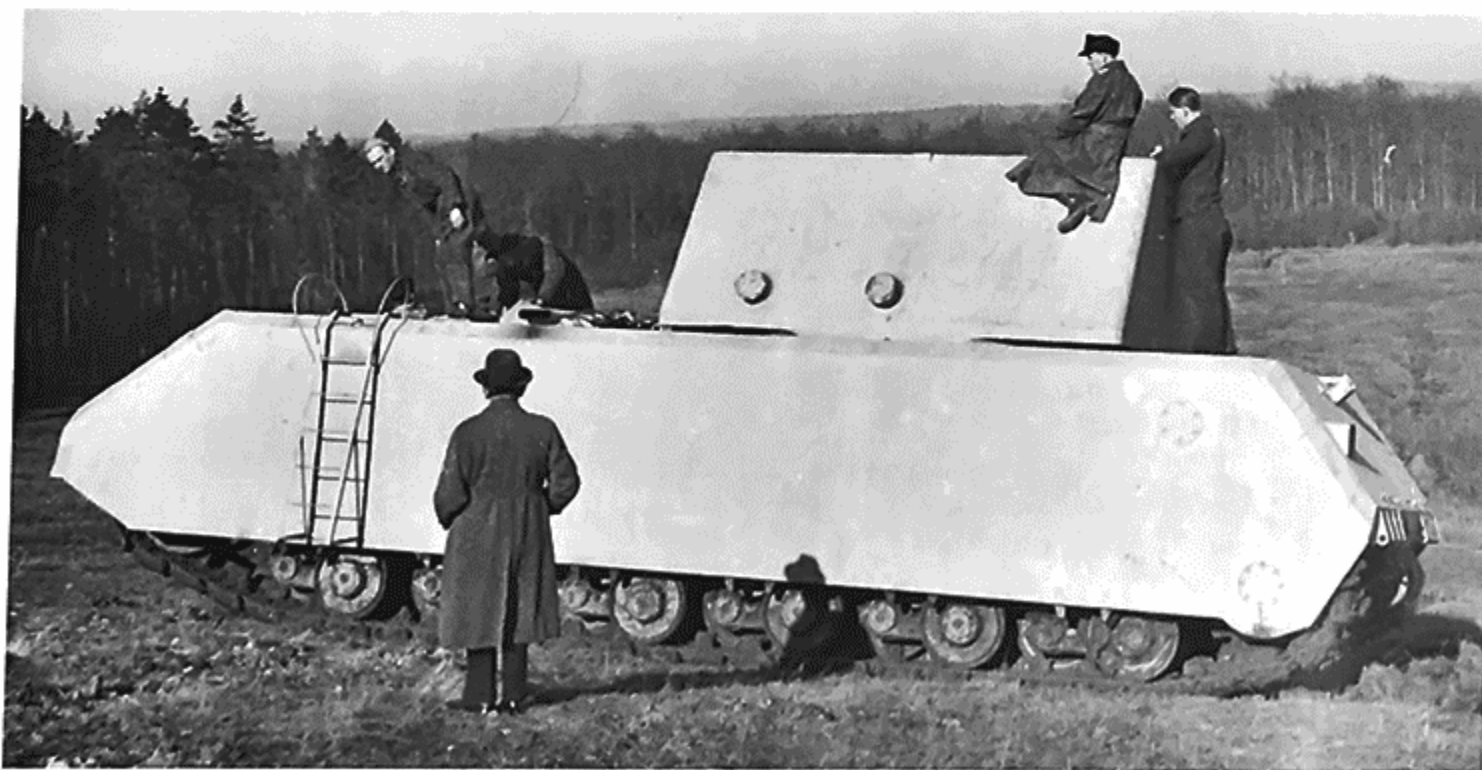
This and Opposite Page: The 1.Maus Versuchs-Fahrgestell (trial chassis) with the Turm-Ersatzgewicht (turret substitute weight) being test driven at Boeblingen with Prof. Dr. Porsche looking on. (TTM)
