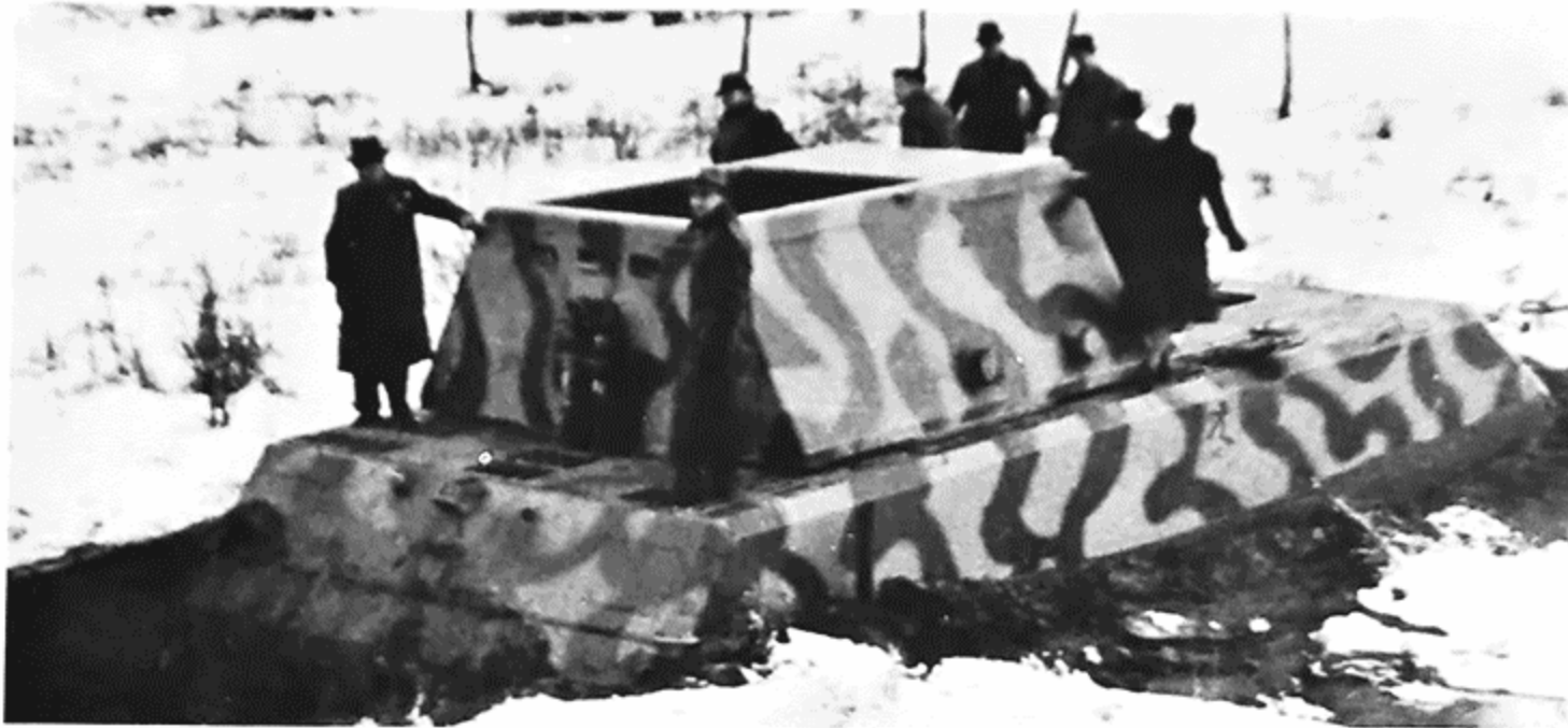
Above and Below: The I.Maus chassis became stuck during a trip through a swampy area because the driver didn't know the area (a region avoided by lighter Panzers). After the mud churned up at the rear was dug out and timbers laid under the tracks, the Maus pulled free under its own power. (TTM)
