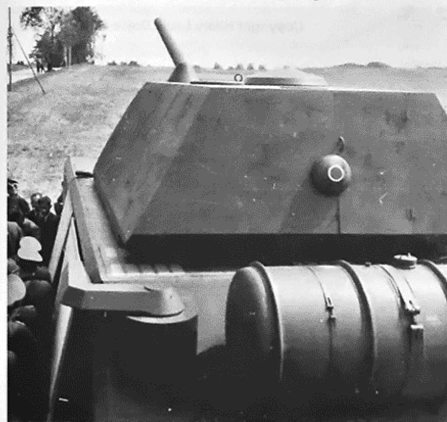
Above Right and Left: The full-scale wooden model of the Porsche-Maus on display for Hitler and entourage on 14 May 1943 still had a commander's cupola on the roof. In 6 decided that the Flammenwerfer (flame thrower) system (mounted on the right and left upper hull rear) would be dropped. (BSB)
