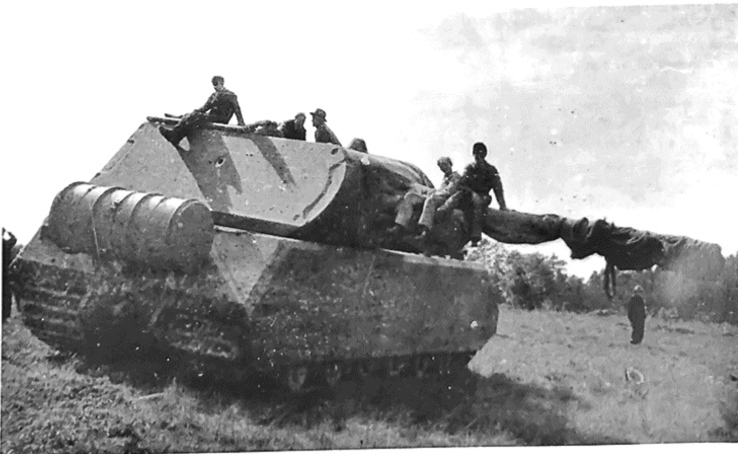
Above and Below: The 2.Versuchs-Fahrgestell with the 1.Versuchs-Turm being test driven at Boeblingen. Holes were drilled in the pressure discs on the roadwheels to prevent the rubber rings from being pushed out of position under the tremendous weight load. (WJS)
