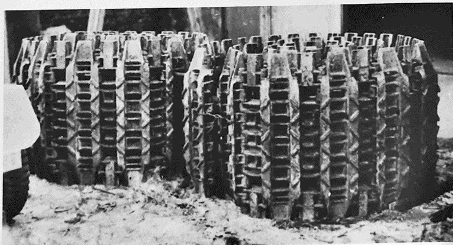
Below: This photograph of the 1000 mm wide Gefechtskette (combat track) was taken after the war. Only the Transportkette (rail transport track) was available in January 1945. (TTM)
